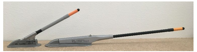
Fig 4. The two dischargers used for the study. Left is the tip null plus discharger mounted to the wing tip, referred to as the angled wick; Right is the null plus trailing edge discharger mounted to the trailing edge of the wing, referred to as the horizontal wick.
